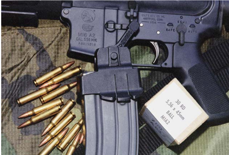
Maglula individual magazine charger in position for loading. (Source: Charles Q Cutshaw)
